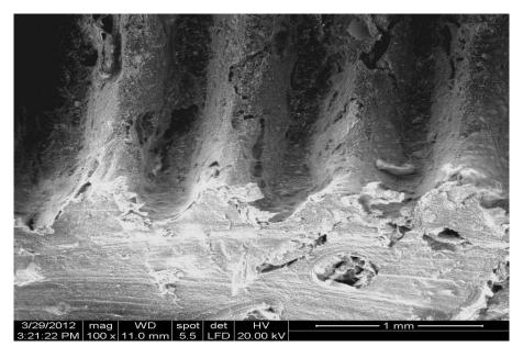
Figure 2. Scanning electron microscopy of the contact zone of bone tissue with a titanium implant (3 months)
