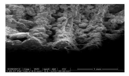
Figure 1. Scanning electron microscopy of the bone tissue contact area with the titanium implant (1 month)
