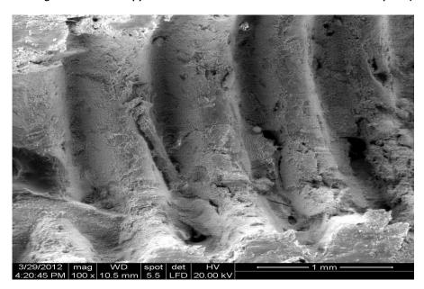
Figure 3. Scanning electron microscopy of the bone tissue contact area with the titanium implant (6 months)
